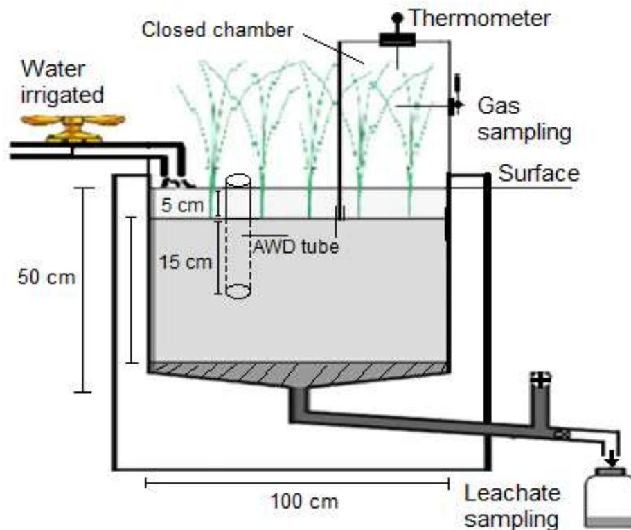
**Figure 1.** Schematic of free drainage lysimeter bucket with closed chamber method.
