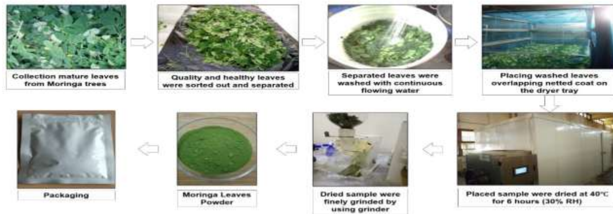
Figure 1. Production process flowchart of moringa leaves powder.
